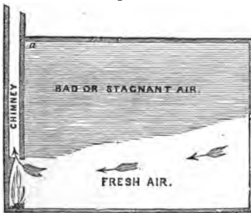
A badly-ventilated Room.
