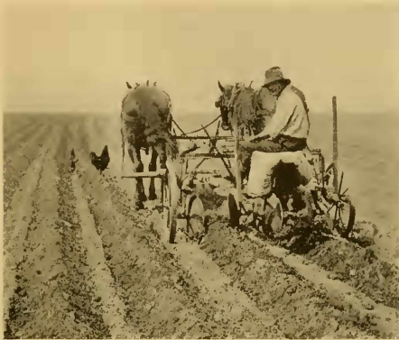
FIG. 41.—A riding 2-row disk horse-hoe ridging or moulding the soil over the plants. This implement requires only one man to operate it.
