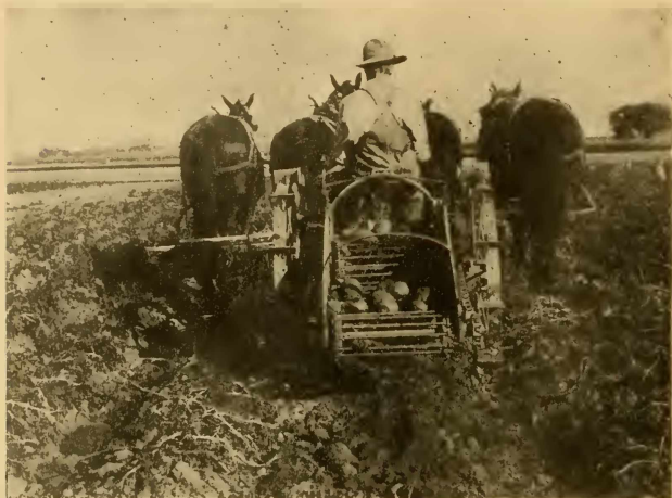
FIG. 81.—A potato digger with rear conveyor belt. Such a machine does not separate the vines from the tubers. Greeley, Col.
