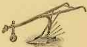
FIG. 72.—The Eclipse digger with rigid rods to separate the tubers from the soil.
