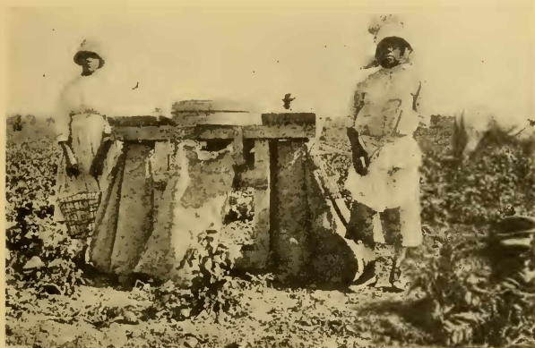
FIG. 90.—Type of hand-sizing screen and stand used in the Eagle Lake district in Texas.
