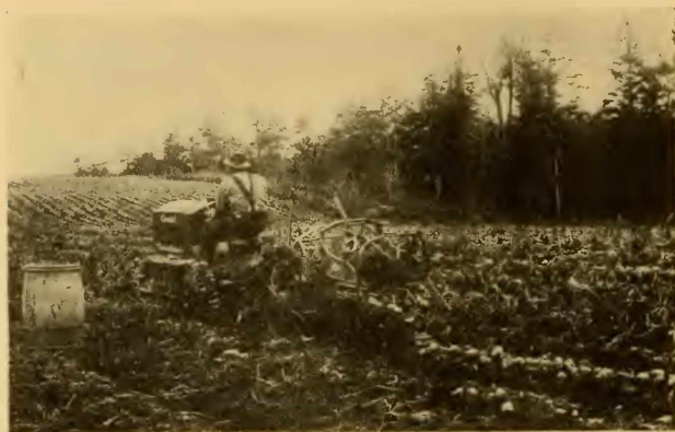
FIG. 83.—The potato digger can be successfully operated by a tractor. Presque Isle, Me.
