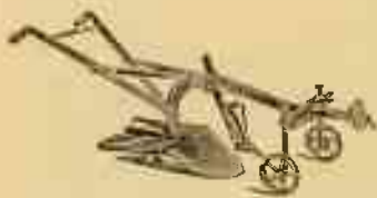
FIG. 73.—A bar type of digger with a sprocket wheel behind to shake the soil from the tubers. The two lead wheels straddle the row.
