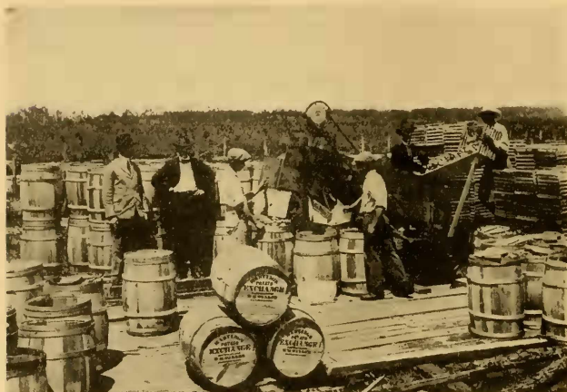
FIG. 87.—Sizing potatoes with a large power-driven sizer having a capacity of over 100 barrels per hour. The potatoes are hauled from the field to the sizer in slat crates. On the G. W. Waller farm, Hastings, Fla.
