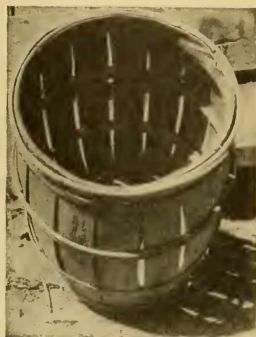
FIG. 96.—The Beaufort S. C. type splint barrel with inner set of hoops which impart a considerable degree of rigidity to the barrel.
