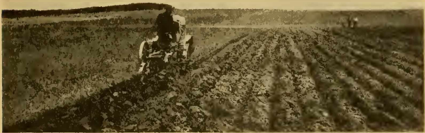
FIG. 7.—Plowing a clover sod with a tractor turning two furrows 14 inches in width and 9 and 10 inches in depth. Aroostook Co., Me., Aug., 1917.
