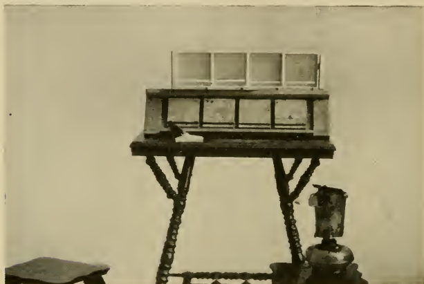
FIG. 74.—The Pangburn foundation fastener and sections filled with foundation.
