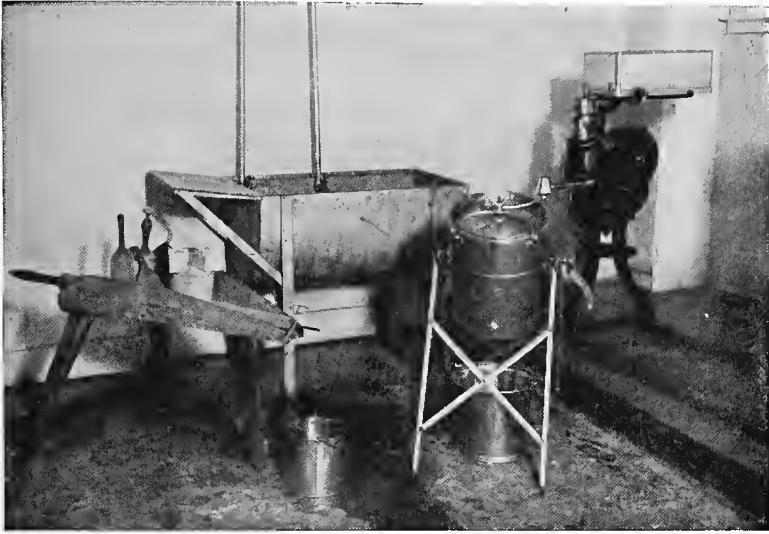
FIG. 116.—Cream separator churn and butter worker suited to the needs of the small dairy.
