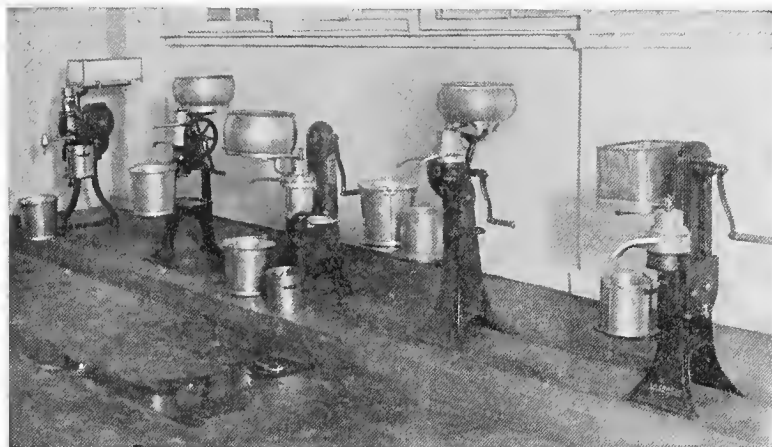
FIG. 112.—There are many makes of hand cream separators having value. This illustrates a few of those used at the Minnesota School of Agriculture.
