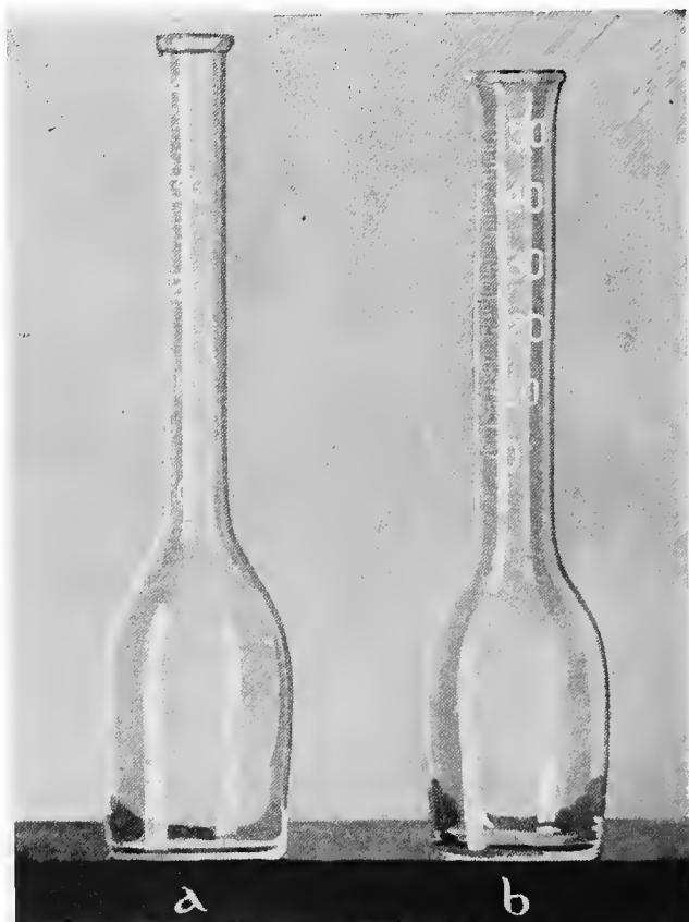
FIG. 108.—Cream test bottles. a is preferable to b in three points. The narrower neck permits more accurate reading of the fat, the neck is straight, i.e. , not flaring toward the top, and the shoulders are more sloping.
