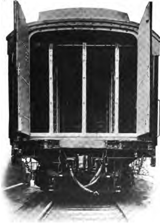
FIG. 166.—Express horse car partitioned into stalls, four groups of four stalls each lengthwise of the car.
