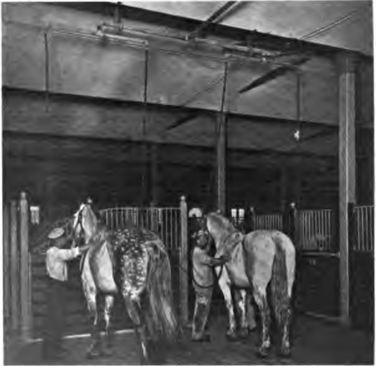
FIG. 134.—A vacuum grooming machine in operation. A vacuum is maintained in the pipes which draws the dirt out of the hair and conveys it to a receptacle where it collects and can be removed.
