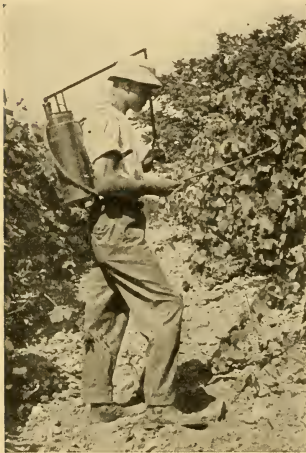
FIG. 77.—Knapsack sprayer. This is an excellent pump for rough ground or where-soever it is difficult to get about, but is rather heavy when one has much spraying to do.
