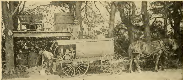
FIG. 82.—A gasolene power outfit. The most efficient power sprayer. The cut also shows an excellent arrangement for filling the tank and mixing the materials.
