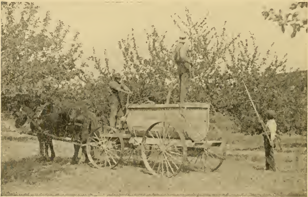
FIG. 80.—A large, double-action, hand pump with 200-gallon tank. An excellent outfit, but it is a man's job to do the pumping.
