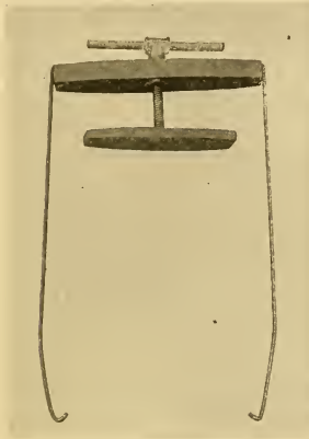
FIG. 126.—The ordinary barrel press with a bar follower. This is not nearly so good as the press shown in Figure 127.
