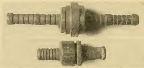
FIG. 86.—Long- and short-tailed hose couplings. The former are much to be preferred, as they do not allow the hose to pull apart so easily.
