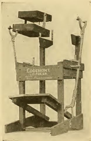
FIG. 140.—A western type of box press.
