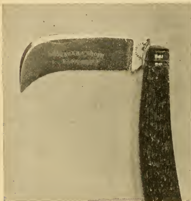
FIG. 64.—A good type of pruning knife. Long hooked blade and large enough for heavy work.
