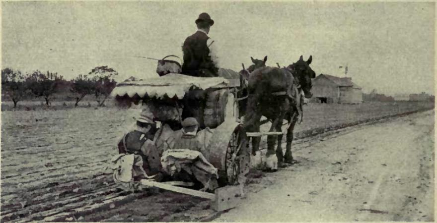
FIG. 255.—Machine at work setting tobacco plants in the open field. The boys behind place the plants in the planting pocket one at a time. The machine opens the furrow, waters the plants, and presses in the soil around them. (U. S. D. A.)
