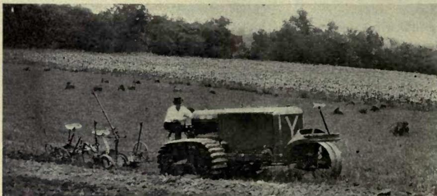
FIG. 70.—This tractor has wheels of the "caterpillar" type and may be used on rather rough land without difficulty. Tractors give enough power to allow very deep tillage of soils. Farming thus becomes both more intensive and more extensive.
