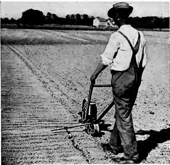
FIG. 44.—Garden seed drill in operation.
