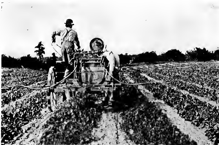
FIG. 52.—Spraying muskmelons with three-row, geared-power sprayer.
