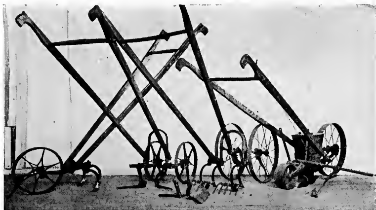
FIG. 102.—Tools used in onion culture: Seed drill at right; double and single wheel hoes with various attachments.
