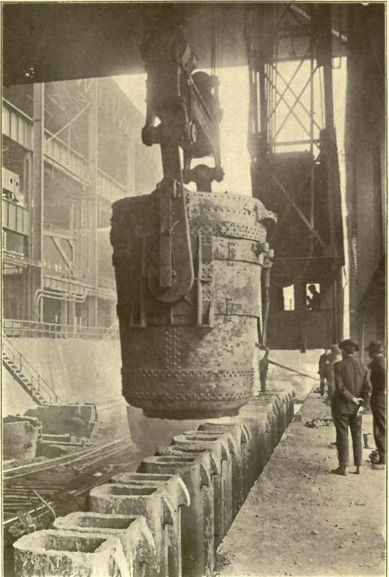
TEEMING A HEAT IN THE OPEN HEARTH DEPARTMENT—SHOWING THE 100-TON LADLE USED.
