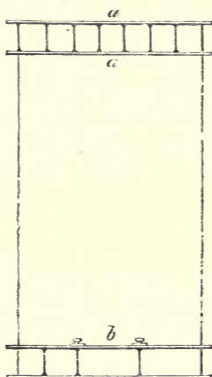
MR. FAIRBAIRN'S FIRST SKETCH FOR THE TUBE OF THE BRITANNIA BRIDGE.
