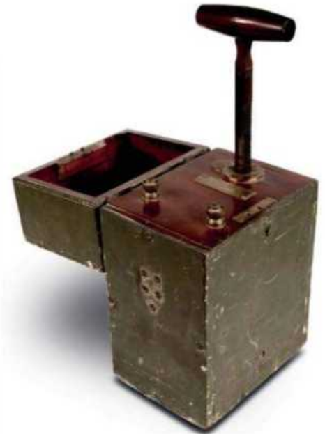
ABOVE: PLUNGING THE HANDLE GENERATED AN ELECTRICAL CHARGE DOWN THE WIRES CONNECTED TO THE TWO KNOBS ON THE BOX AND SET OFF AN ELECTRIC DETONATOR IN THE EXPLOSIVE.
