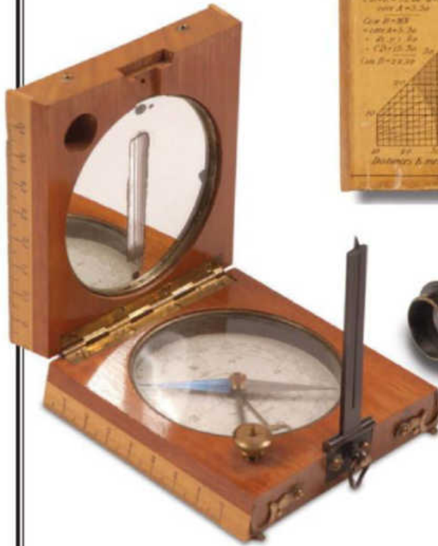
ABOVE: A French artillery officer's magnetic compass. To take a bearing, the observer lined up the object through the slit in the rod and mirror
