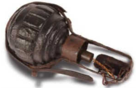
BELOW: German time-fused "ball" grenade. The throwing handle pulled the friction igniter as the grenade was thrown
