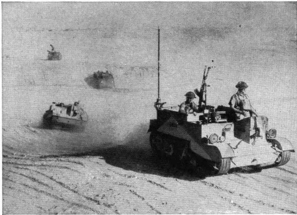
FIGURE 93.—Universal armoured carrier fitted with Bren gun on anti-aircraft mount and with Boys anti-tank rifle.
