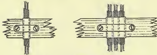
METHOD OF CLEATING ON BATTENS .
