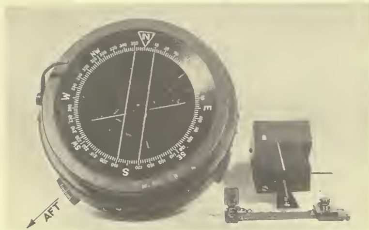
FIG. 67. P-4 COMPASS WITH CORRECTOR BOX DETACHED SHOWING MAGNETS PARTIALLY WITHDRAWN
