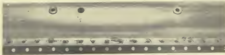
FIG. 16. STRESS AND CORROSION CRACKS IN HIGH-TENSILE STAINLESS STEEL SPAR FLANGE
