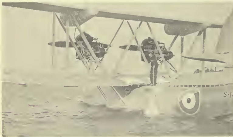
FIG. 53. HAULING DROGUE ON BOARD AFTER AIRCRAFT HAS BEEN MADE FAST AT MOORINGS
