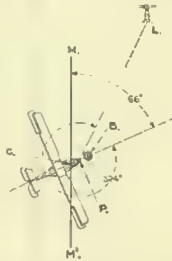
FIG. 69. SWINGING AN AIRCRAFT Afloat BY BEARING PLATE
