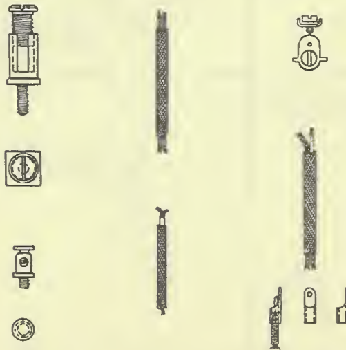
METHOD OF FIXING CABLE ENDS AT TERMINALS.
