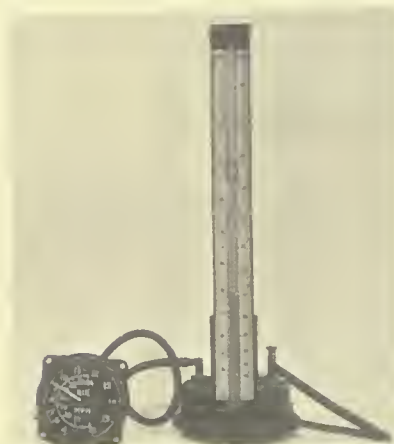
FIG. 59. AIR SPEED INDICATOR UNDER TEST (READING M.P.H.)
