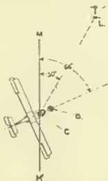
FIG. 68. SWINGING AN AIRCRAFT Afloat BY BEARING COMPASS
