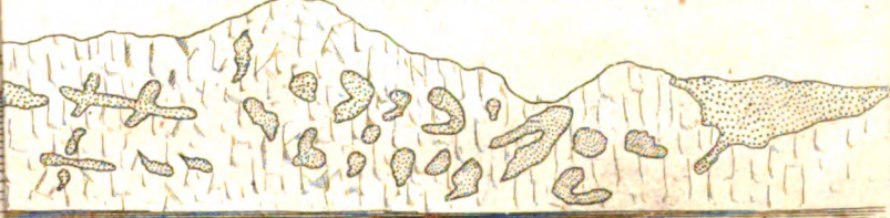
Fig 20. Granite of Roene's Hill traversed by veins of Sienitic Greenstone.
