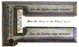
Sketch of the manner in which the Water is filled from the Troughs into the Bucksts
