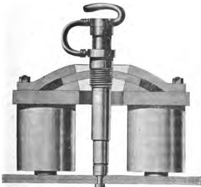
Fig. 11.—Electro-Pneumatic Riveter, with spherical flange attachment for adjusting direction of blows.
