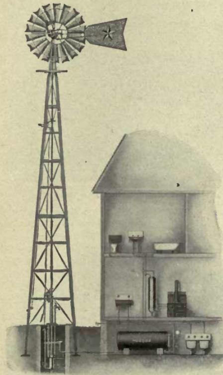
FIG. 310.—Hydro-pneumatic pressure system with tank containing air and water under high pressure. The pressure is maintained with a pump operated by engine, motor, or wind mill. (Flint and Walling Mfg. Co.)
