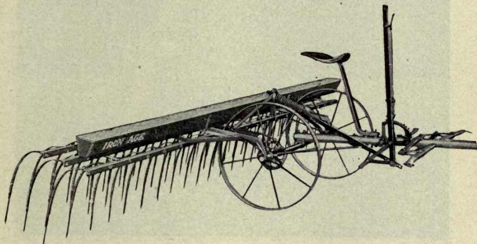
FIG. 68.—The weeder will produce a fine dust mulch and conserve moisture in the soil.
