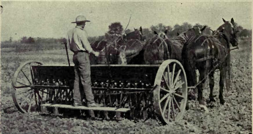
FIG. 150.—Wide grain drill drawn by four heavy horses. It is well adapted to the large farms in the grain belt. (I. H. Co.)
