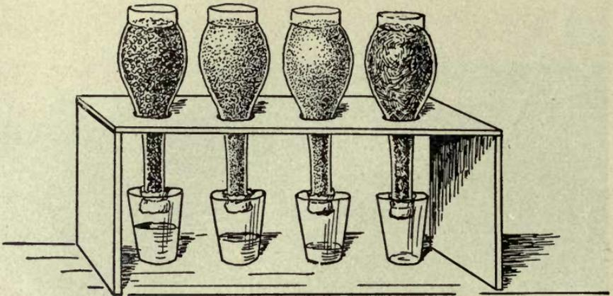
FIG. 65.—Common lamp chimneys with cloth tied on to prevent the escape of soil samples placed in them. This may be used to show the rate at which different soils will take up rain water and their relative power of retaining water for use of crops. From left to right they may contain coarse sand, loam, clay, and humus soil.
