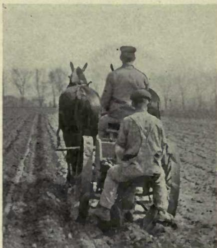
FIG. 162.—This type of planter requires two men to operate it—one drives the team and the other distributes the potatoes in the dropping disk to insure uniform planting. (Bateman Mfg. Co.)
