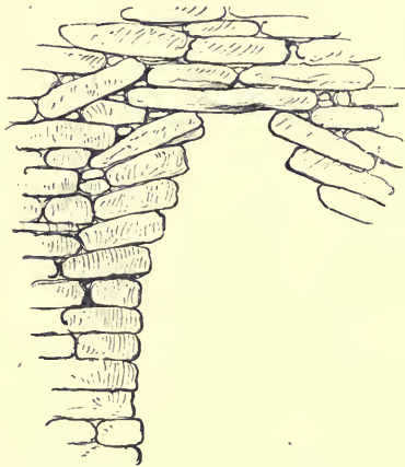
Fig. 190.—Section of Chamber in Broch of Kintradwell, showing rude vaulting of roof. (From a Drawing by Rev. Dr. Joass.)
