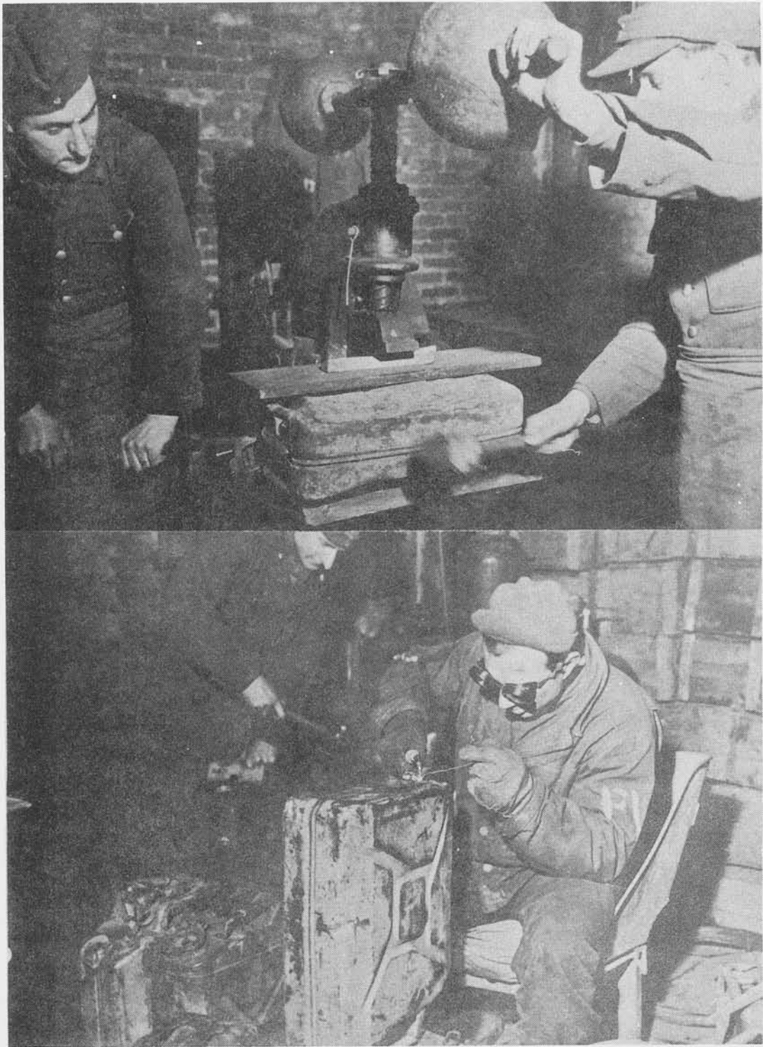
FIGURE 46.—After Dents Were Removed from Jerri-cans with Home-made Jigs and Presses, Holes Were Patched and Seams Were Mended.
