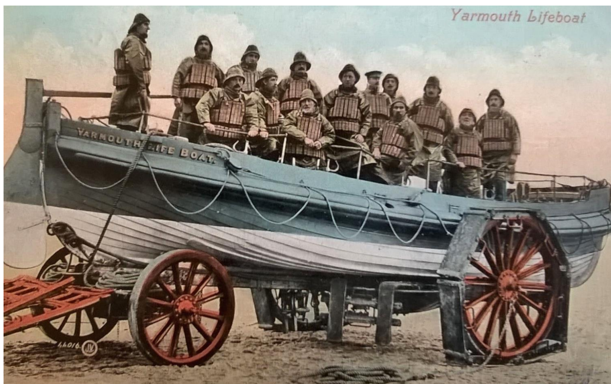
Yarmouth lifeboat, carriage, and crew wearing their cork life-jackets. Note the apparatus fitted to the large wheels to prevent them sinking into the sand.
