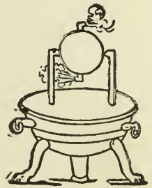
HERO'S ROTATING STEAM-ENGINE.
