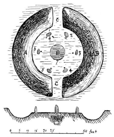
Fig. 200.—Ground-plan and section of stone circle at Crichie.
