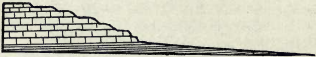
Diagram showing effect on hill outlines of volcanic lavas overlying softer sedimentary rocks
