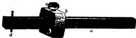
FIG. 15. — Marking gauge. a , bar; b , head; c , thumbscrew; d , point.
