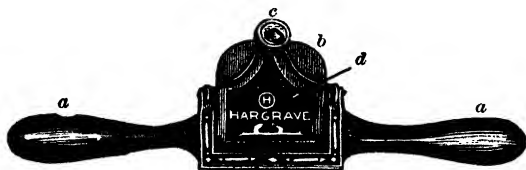
FIG. 43 — Spokeshave. a , handle; b , blade; c , set screw; d , cap iron.
