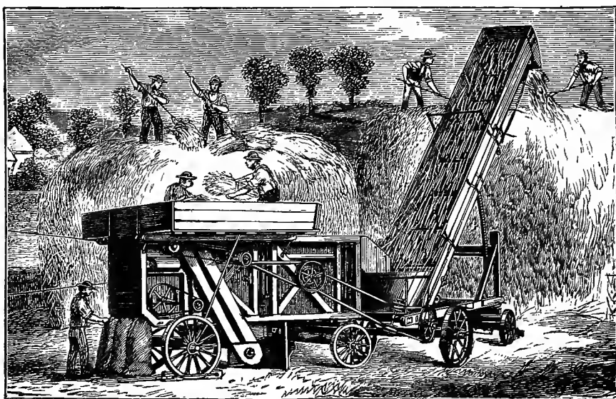
Fig. 174.—Portable threshing-machine, showing straw-elevator.
