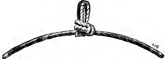
Fig. 518.—Knot tied by the Hornsby binder.
