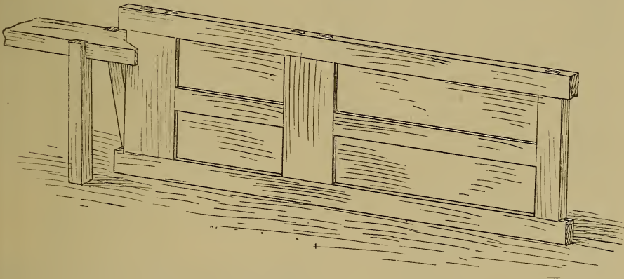
Fig. 1124.—Door in Position for Shooting Edge.
