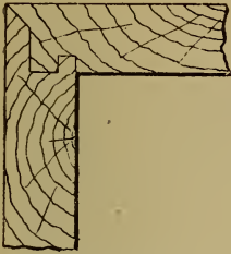
Fig. 272.— Mitred, Grooved, and Tongued Joint.
