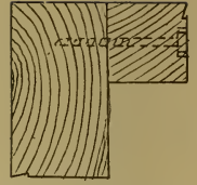
Fig. 712.—Angle Post formed of Two Pieces butting and bolted together.
