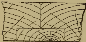
Fig. 379.— Rebated, Grooved and Tongued Joint for Secret Nailing.
