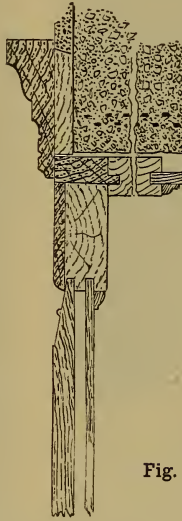
Figs. 1238 and 1239.—Details of Architraves and Top Rail of Door in Section.
