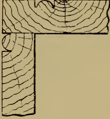
Fig. 277.— Butt Joint with Flush Beads.
