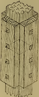
Fig. 235.—Double Fished Butt Joint for Detached Post.
