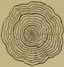
Fig. 163.—Cup-shake in Log.
