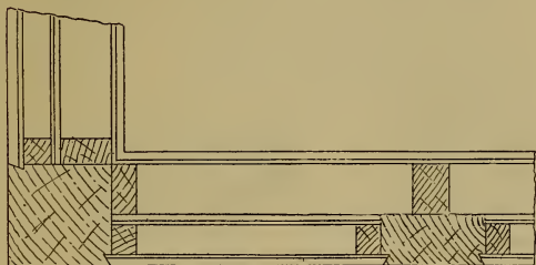
Fig. 709.—Section showing External Stucco, Middle Coat of Lath and Plaster, and Internal Lathing and Plastering.
