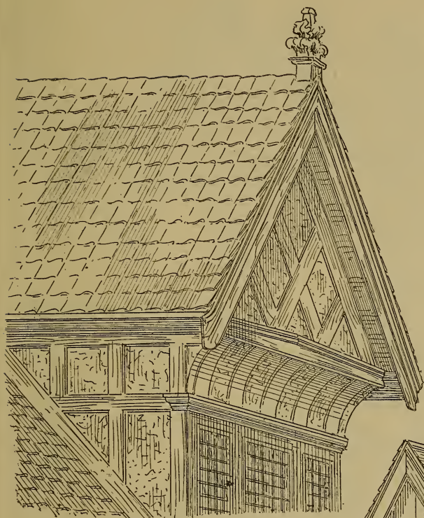
Fig. 736.—Method of finishing Upper Portion of Small Gable.
