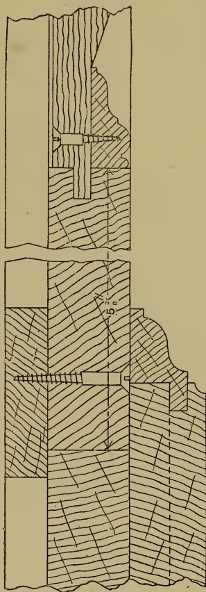
Fig. 1628.—Detail Section of Lower Part of Dado.
