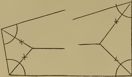
Fig. 614.—Method of Obtaining Positions of Hips.
