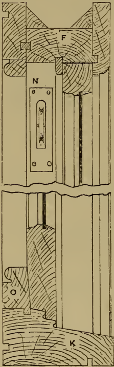
Fig. 1424.—Vertical Section through Head and Sill.
