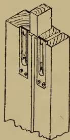
Fig. 1420.—Top of Mullion, showing Pulleys and Tenon.
