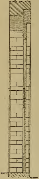
Fig. 1073.—Vertical Section of Stable Doors.
