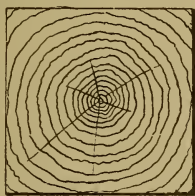
Fig. 169.—Star-shake in Balk.
