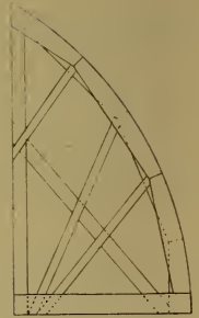
Fig. 935.— Construction of a Secondary Rib.
