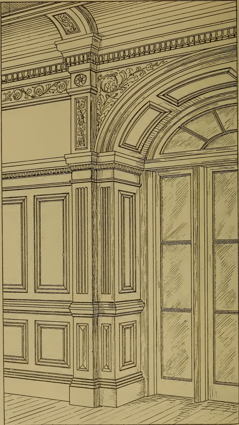
Fig. 1671.—Pilaster, Linings, Soffit, Cove of Ceiling, etc.
