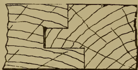
Fig. 380.— Iron Tongue Joint.
