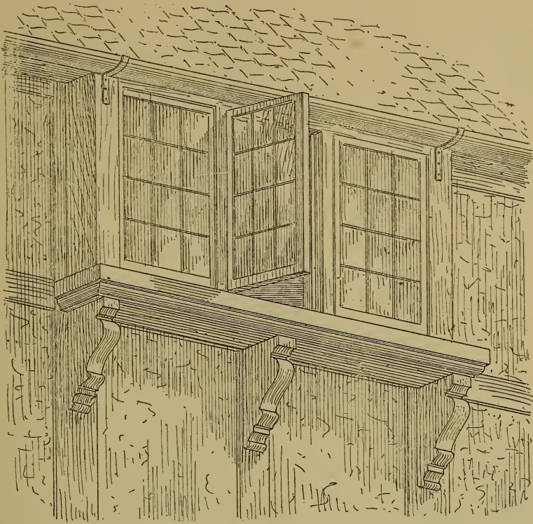
Fig. 733.—Conventional View of Projecting Window supported on Moulded Brackets.
