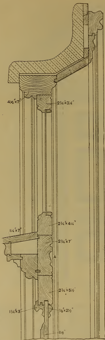
Fig. 1260. — Enlarged Detail of Upper Part of Vertical Section (Fig. 1258).
