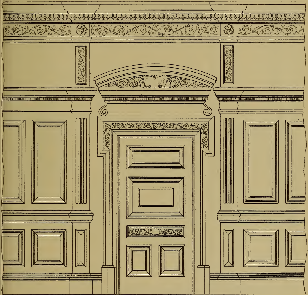
Fig. 1668.—Elevation of Door and Portion of Panelling.
