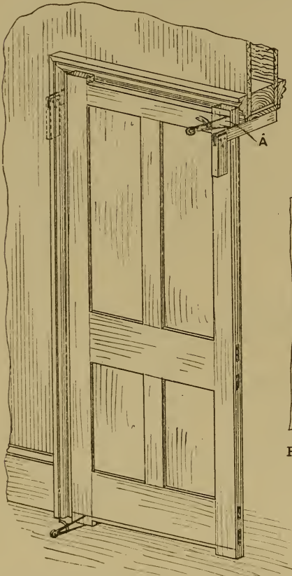
Fig. 1125.—Scribing Door for Height.
