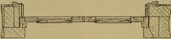
Fig. 1225.—Horizontal Section of Double-margin Door.
