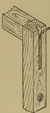
Fig. 1381.—Attaching Cord to Sash by a Knot.
