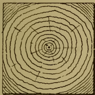
Fig. 167.—Sapwood in Balk.
