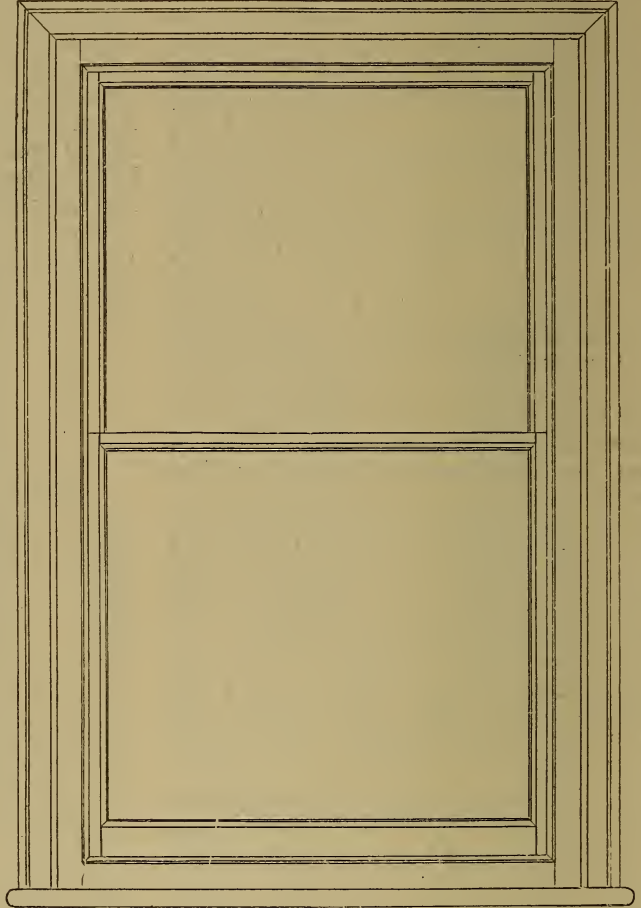
Fig. 1385.—Elevation of Double-Hung Window.
