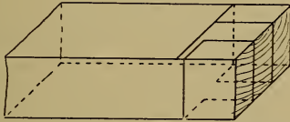
Fig. 1041.—Setting Out Head for Mortices.
