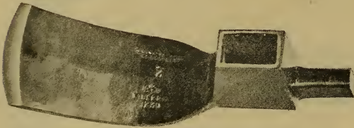
Fig. 96.—Scotch Adze Head.
