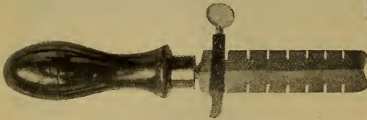
Fig. 86.—Saw Set with Gauge.
