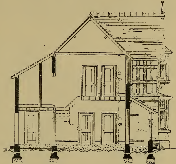
Fig. 724.— Sectional Elevation of Half-timbered House.
