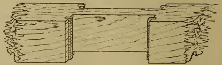
Fig. 1227.—View of Top Rail prepared to receive End of Centre Stile.
