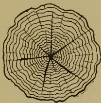
Fig. 168.—Star-shake in Log.
