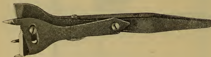
Fig. 109.—Anderson's Expanding Bit.
