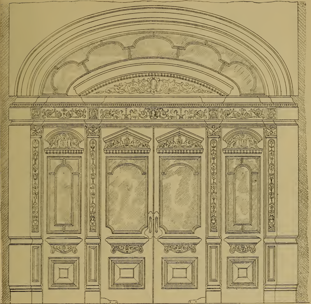
Fig. 1726.—Outside Elevation of Vestibule Framing with Swing Doors.
