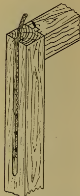
Fig. 1382.—Attaching Cord to Sash by Nails.
