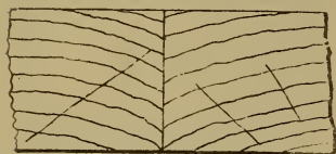
Fig. 377.— Rebated Floor Joint.
