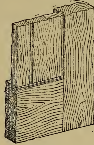
Fig. 1070.—Conventional Detail of Corner of Door at A, B, C (Fig. 1065).
