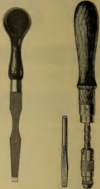
Fig. 97.—Plain Handle London Screwdriver.
