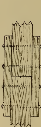
Fig. 234.—Single Fished Butt Joint when Post is Braced.
