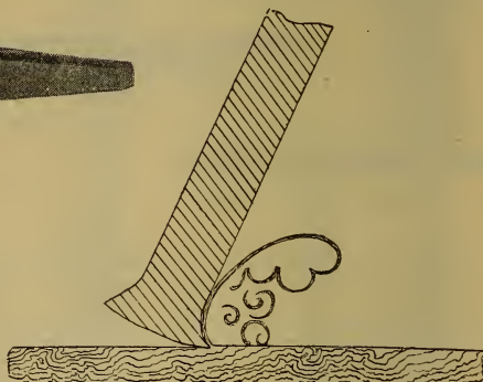
Fig. 113.—Action of Steel Scraper.
