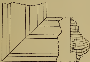
Fig. 151.—Best Arrangement of Grain in Mouldings.
