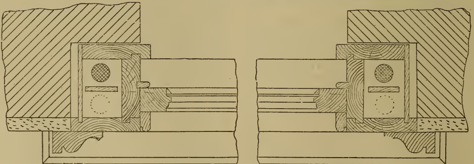
Fig. 1386.—Horizontal Section of Double-Hung Window.
