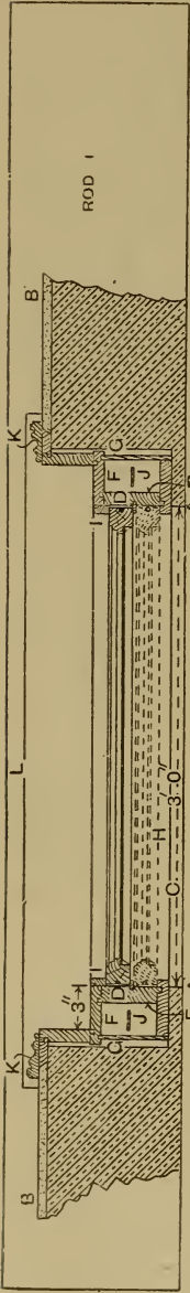
Fig. 951.—Width Rod showing Plan of Sash Frame.
