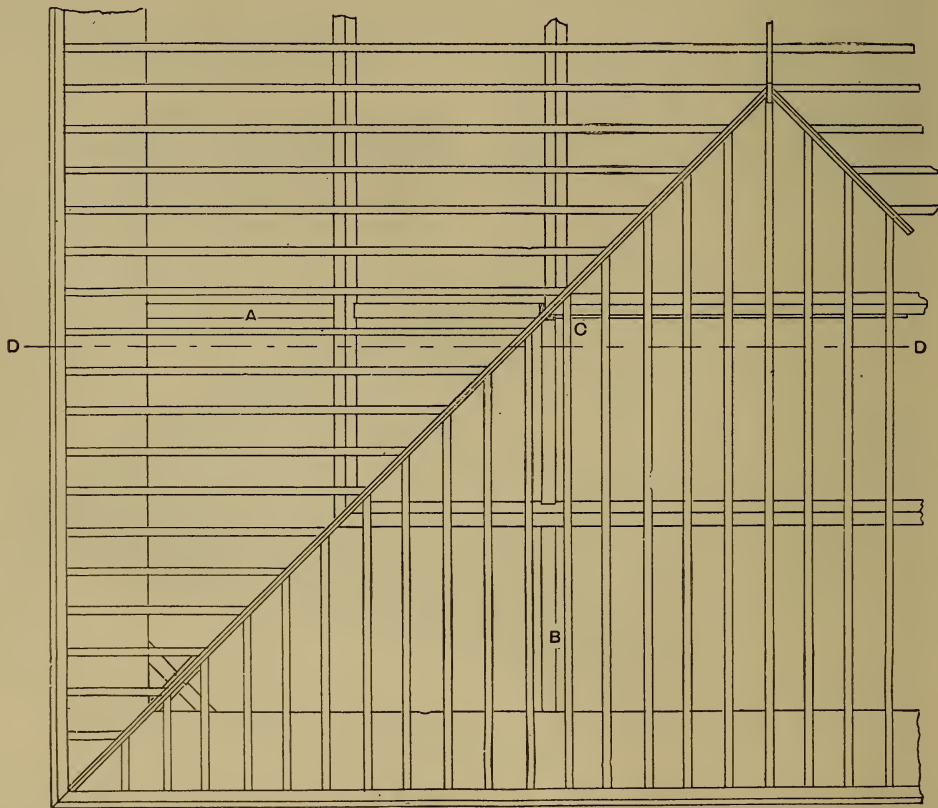
Fig. 489.—Part Plan of Queen-post Truss with Hipped End, showing Timbers—A, Main Truss, B, Half Truss, both being connected at C.
