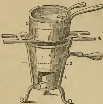
Portable French Furnace, with Stewpan and Trevet.
