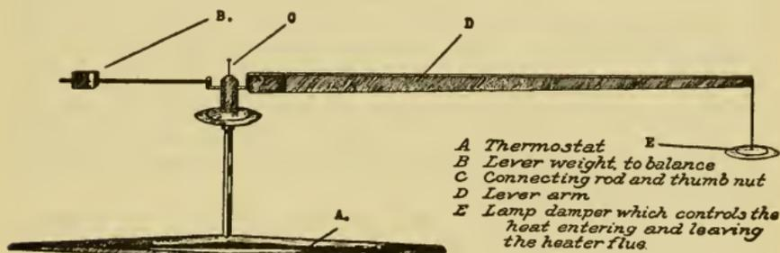
FIG. 159.—A complete self-regulating device for incubators heated by lamps.
