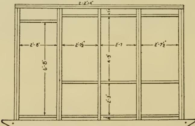
FIG. 92a.—Portable laying house: Working plans.
