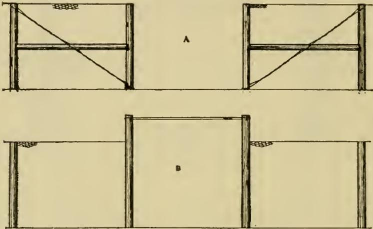
FIG. 111.—Ways of bracing gate posts. A, By using next post in line, similar to corner bracing; B, by overhead wire, especially useful with narrow gates.
