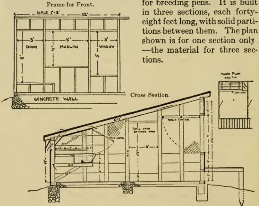
FIG. 86.—Working plans of small-unit laying house. (See text for description.)
