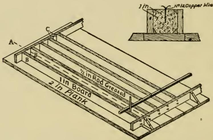
FIG. 108.—Forms for making concrete fence posts.
