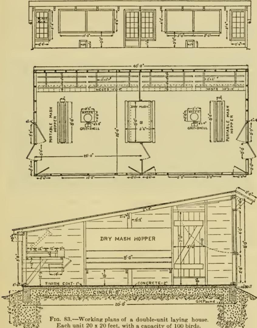
FIG. 83.—Working plans of a double-unit laying house.
