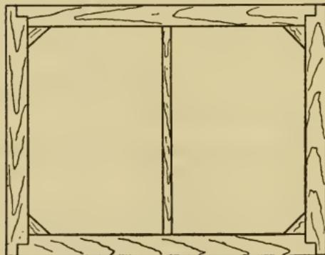
FIG. 78.—Two plans for constructing frames for muslin curtains.
