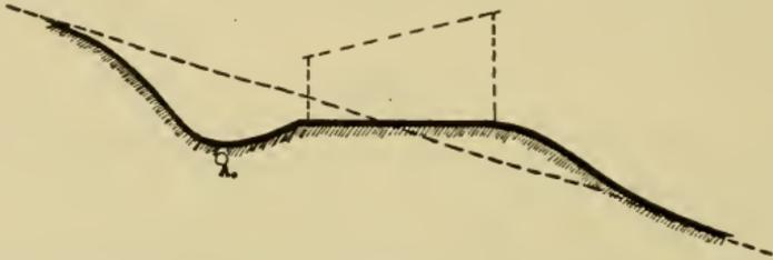
FIG. 79.—Cross section of hillside, showing manner of grading before laying out foundation. The long dotted line shows original slope and the heavy black line shows the surface graded for the poultry house. The house is shown in outline. Drain tile may be placed at *a* to carry water below the house.
