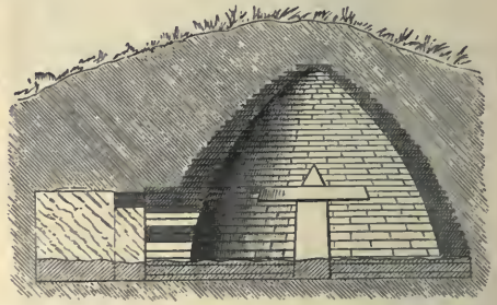
Fig. 11.—Section of Tomb of Atreus at Mycenæ.
