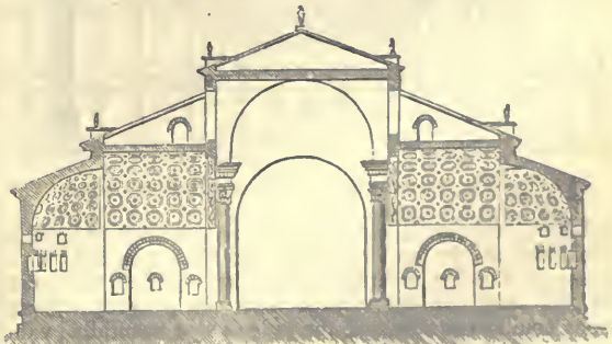
Fig. 22.—Transverse Section of Basilica of Maxentius. (From Fergusson's Hand-book of Architecture .)
