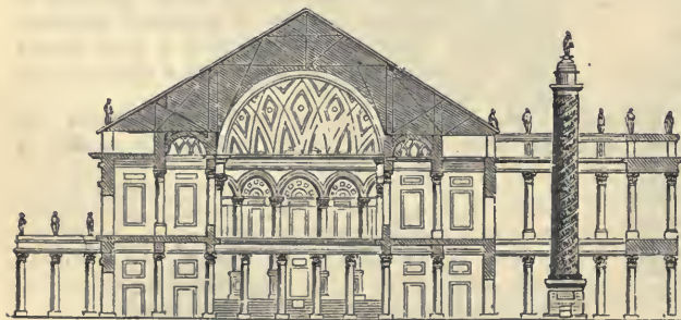
Fig. 23.—Section of Trajan's Basilica, Rome.
