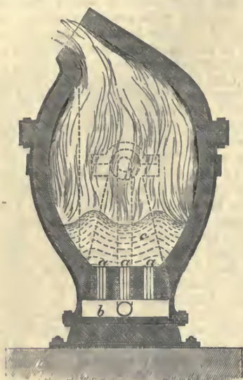
Fig. 6.—Bessemer Converting Vessel : a, a, a, tuyères; b, air-space; c, melted metal.
