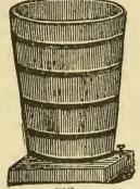
Fig. 1 represents the downward method as employed in the Kedzie filter, manufactured in Rochester, N. Y. The water is poured in at the top and drawn off through the faucet at the bottom. this method the impurities are all retained as the water is passed through, and the material soon be-
