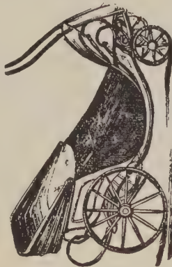
No. 17 is a four-wheeled Victoria Pleasure Ground Chair, mounted in a very light iron framed carriage, upon c and patent India-rubber springs, is either drawn by hand or animal, and is the most elegant and easiest chair made.
