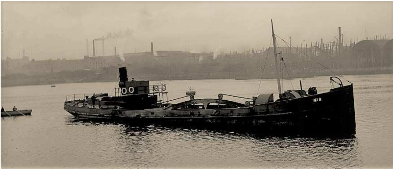
Typical hopper barge. (Photographer unknown).
