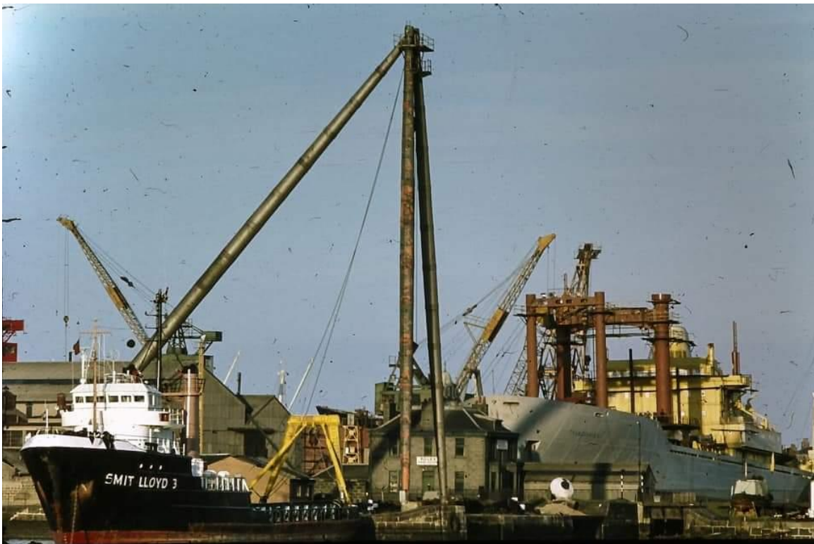
100-ton Shear Poles , the vessel in the background berthed at Hall Russell's Outfitting Quay is the ' Thameshaven ' (8,992 tons), she was the biggest vessel ever launched in Aberdeen. Looks like the Shear Poles are soon to lift a relatively small offshore structure onboard offshore supply vessel ' SMIT LLOYD 3 '. (Douglas Winton, 1971).
