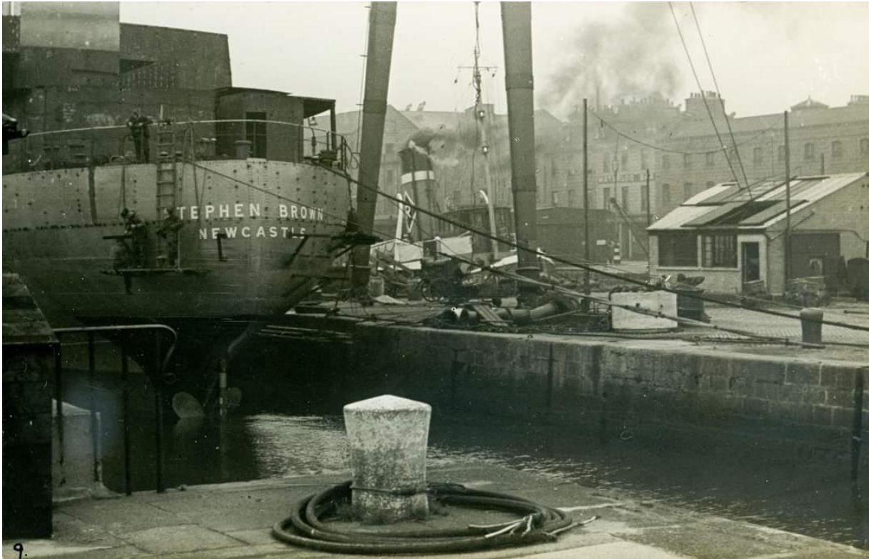
The collier 'Stephen Brown' (1,464 tons) built by Hall, Russell & Co., Ltd. berthed at the 100-ton Shear Poles in 1954 to get her machinery installed. (Photographer unknown).
