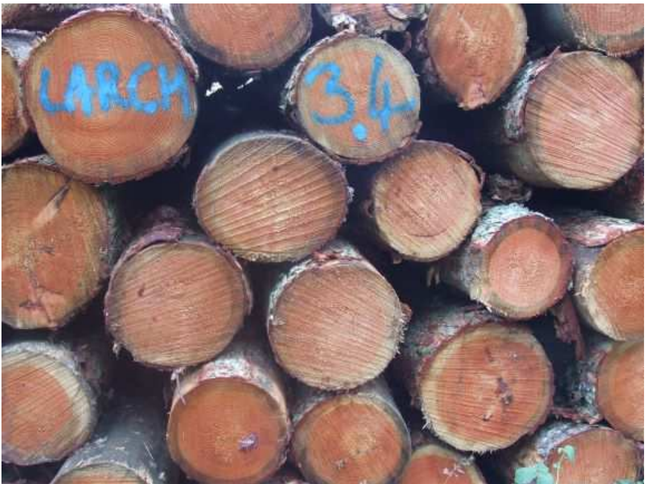
Typical stack of cut Scottish Larch (softwood) timber. (S. Bruce).
