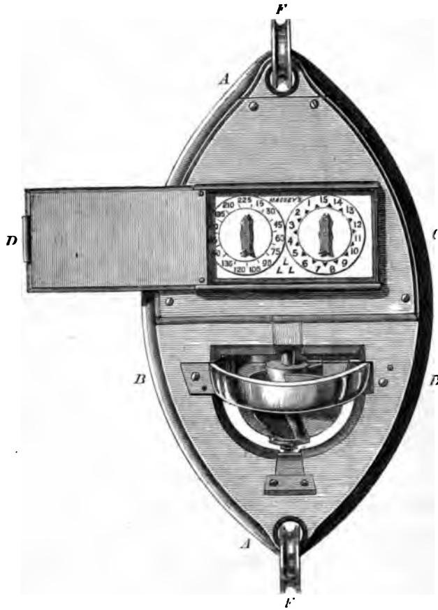
FIG. 43.—'Massey's' Sounding Machine.
