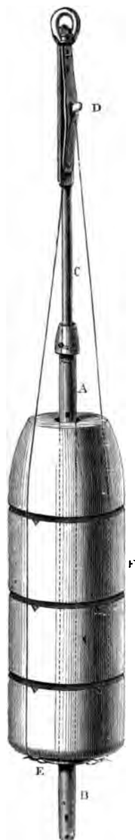
FIG. 42.—The 'Hydra' Sounding Machine.
