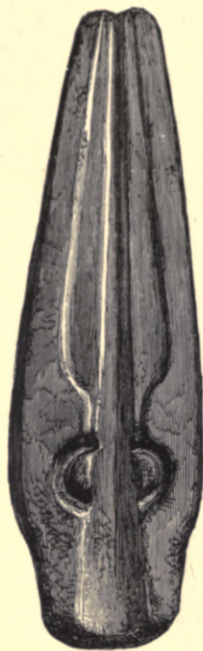
Fig. 196.—Half of a Stone Mould for casting Bronze Spear-heads (7 inches in length).
