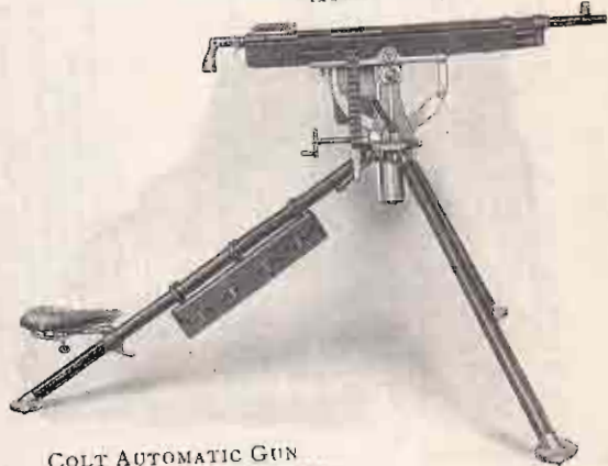
COLT AUTOMATIC GUN MOUNTED ON TRIPOD, SHOWING BELT PASSING OUT ( Right Side ).
