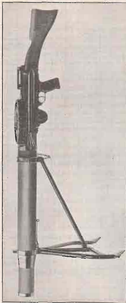
GUN COMPLETE, WITH MAGAZINE AND LIGHT FOLDING FIELD MOUNT.
