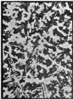
Fig. 25. White Cast Iron as Cast. M.S. tons per square inch, 22·8.
