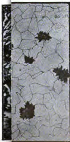
Fig. 20. Microstructure of special cast iron (known as black heart). Magnification 90 dias.
