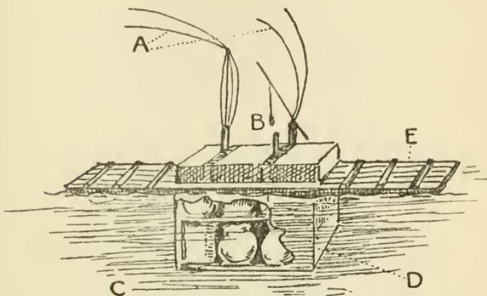
A, Wires to catch side of ship. B, Lead weight. C, Jars of Gunpowder.
