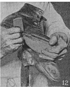
Boot Repairing. Figs. 10-15. Concluding stages in soleing and heeling a pair of boots, showing how the heels and soles should be finished off with a rasp and sandpaper and finally burnished.
