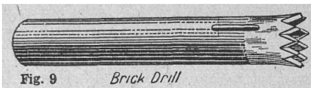
Drill. Fig. 9. Diagram of drill made from iron gas barrel, for brickwork.
