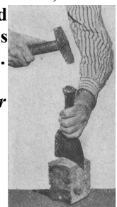
Brick. Fig. 9. Bricklayer's bolster for cutting and shaping bricks.
