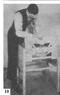
Gramophone. Fig. 8. Console gramophone cabinet. Fig. 9. Assembling the main framework. Fig. 10. Sliding the front fret into position. Fig. 11. The horn being fitted into the centre compartment beneath motor board.
