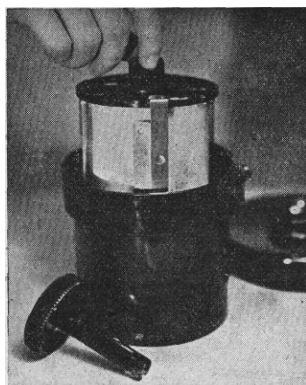
Fig. 4. Film and apron, secured by clip, is dropped into tank. The components (see text for details).
