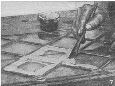
Fig. 7. Brushing cement into joints with an old paint brush.
