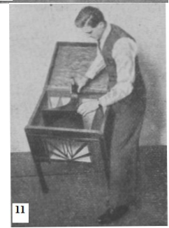
Gramophone. Fig. 8. Console gramophone cabinet. Fig. 9. Assembling the main framework. Fig. 10. Sliding the front fret into position. Fig. 11. The horn being fitted into the centre compartment beneath motor board.
