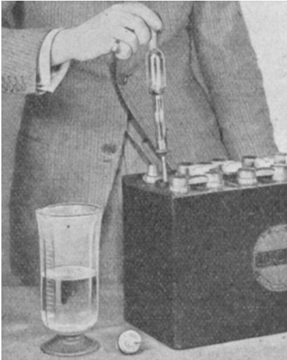
Accumulator. The state of the battery should be tested with the hydrometer, and distilled water added if the plates are not well covered.
