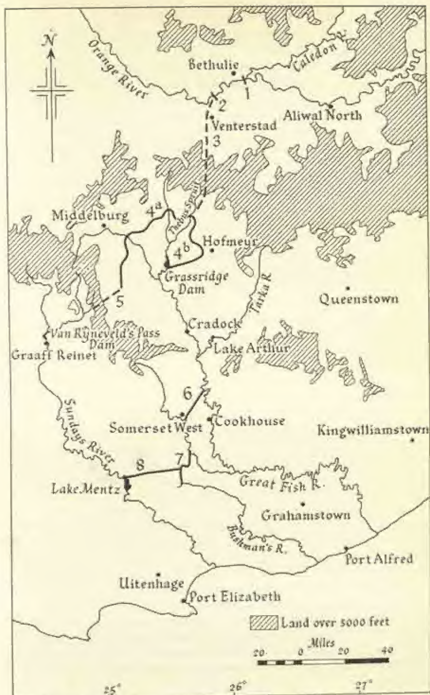
Fig. 55. The scheme for the diversion of water from the Orange river into the Great Fish and Sundays river valleys.
