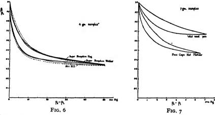
close together. The areas of the loops when measured in arbitrary units by a planimeter are Super Shropshire hog 21.1, Super Shropshire wether 22.6 and 50's N.Z. wether 30.2. The first two are so close that the difference probably lies within the experimental error of the method, but there is no doubt they are both more resilient than the 50's N.Z. wether.
