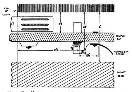
Fig. 1. Plan of Loom mountings shown in Plate II. Measurements indicate approximate relationships of mountings to fell of cloth.
