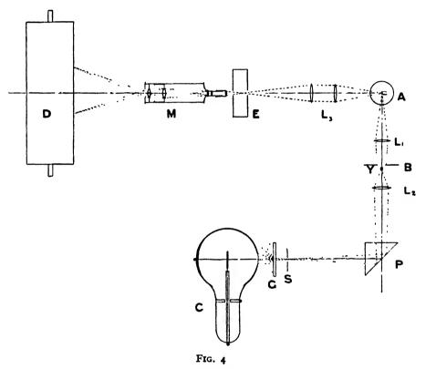
Diagrammatic View of Photoelectric Levelness Tester.
