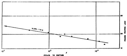
GRAPH. I.—Relation of Cycles-to-Rupture to Pounds wearing Load in Preliminary Test with modified Amsler Wear Testing Apparatus.
