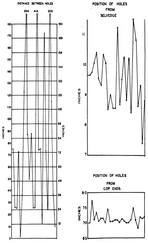
Fig. 4. Pink Limbric: Series of Graphs definitely indicating conditions produced by "shuttle-tapping."
