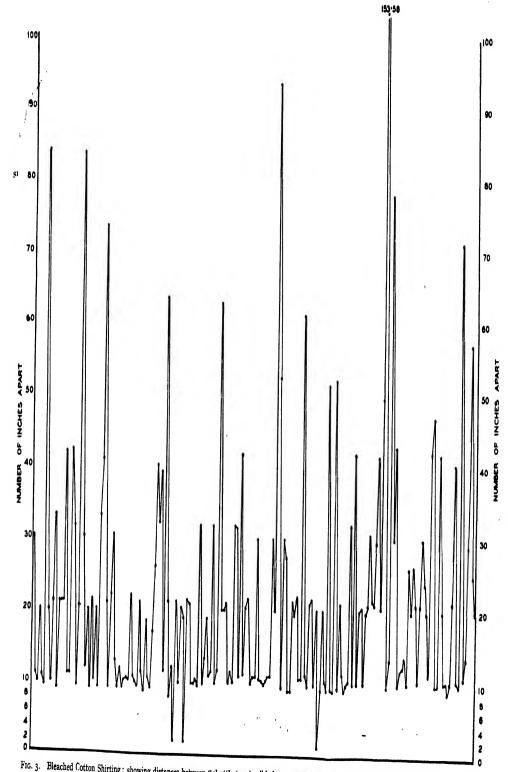
Fig. 3. Bleached Cotton Shirting: showing distances between "shuttle-tapping" holes, measured warp-way. Average length woven by full cop—10 inches.
