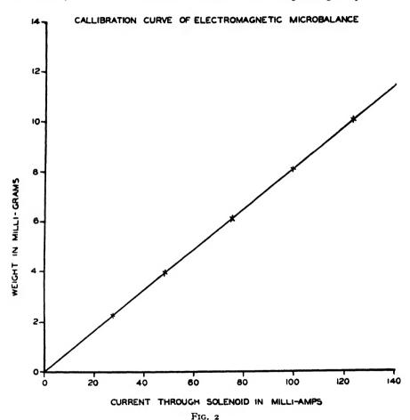
Curve showing the Relation between Weight and Solenoid Current for the Electromagnetic Microbalance.
