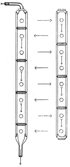
Fig. III (b). Diagram of mercury seal units; the sample containers are not shown, but the direction of the air current through them is indicated by arrows.
