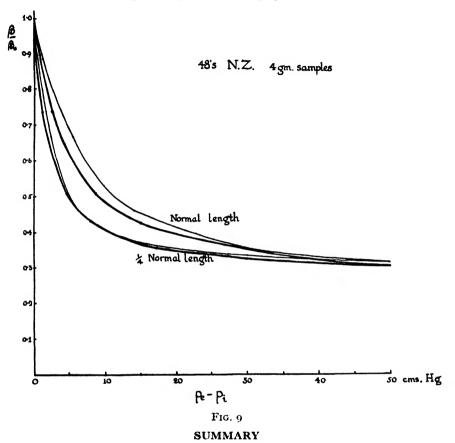
An attempt has been made to measure the resilience of a volume of wool by enclosing it in a thin spherical rubber membrane and submitting it to the mechanical action of a surrounding atmosphere whose pressure is made to vary in a cyclic manner.
