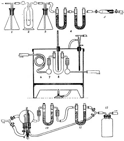
Fig. 1II (a). Diagram of Drying Apparatus: (1), cotton-wool filter; (2), sulphuric acid container; (3), glass-wool filter; (4), CaCl<sub>2</sub> drying U-tubes; (5), P<sub>2</sub>O<sub>5</sub> tube; (6), lead pipe coil; (7), mercury seal; (8), wool sample container; (9), indicator-condenser; (10), CaCl<sub>2</sub> U-tube moisture indicator; (11), CaCl<sub>2</sub> tube to prevent diffusion of moisture back from pump; (12), water trap.
