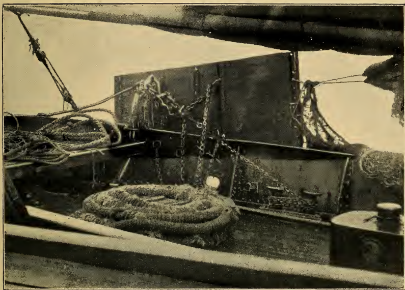
Wing of otter-trawl at stern of ship. The chain and block passing obliquely from the right is for hoisting. The cod-end of the net, with a rubbing-piece, is tied to the wing (for drying) on the upper right.
